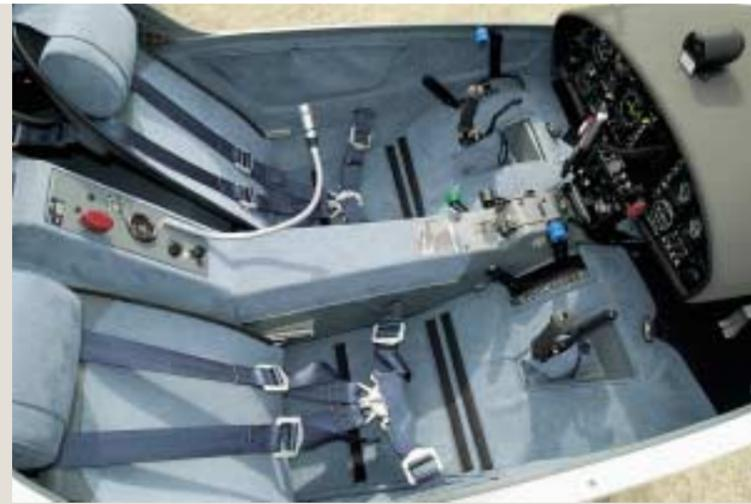
The **cockpit** is a carbon fibre shell, kevlar-lined for impact safety. Inside width is 1.15 meters (3 ft 9 1/4 in) and the one piece canopy hinges from the front with supporting gas springs. The seat backs have six mounting positions, and are further adjusted for angle.
