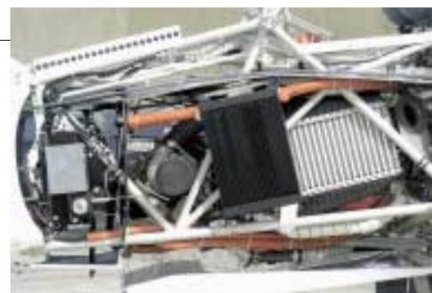
Turbo-oil cooler - intercooler (from left to right)
