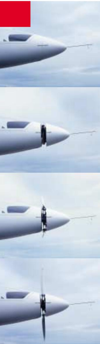
The propeller blades extend into the airstream automatically by centrifugal force when the engine is started.
