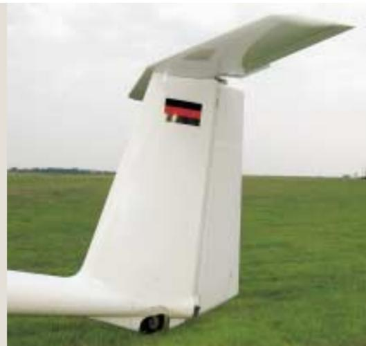
The "T"-tail has a **dampened elevator**, and the rudder size is ample for good control coordination.
