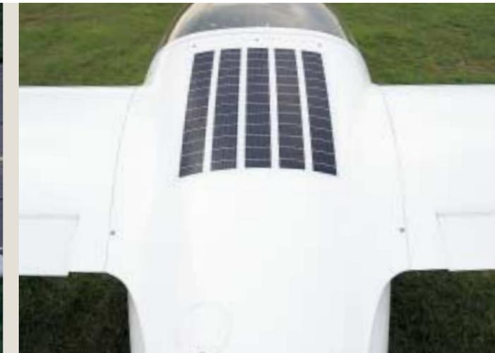
**Solar panels**... providing you with over 30W electrical power during your soaring flight.
