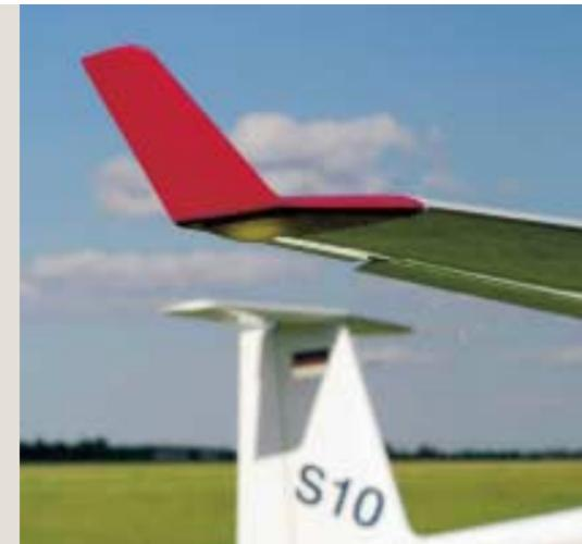
Optional, removable **winglets** improve again the excellent flight characteristics when thermalling, and diminish the sink rate without impairing the spectacular gliding performance in straight flight.
