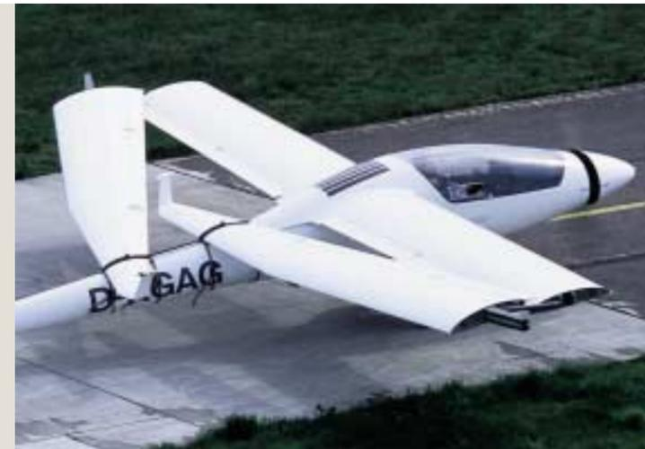
An optional **wing folding system** for taxiing, service, refuelling and lower hangar cost.
